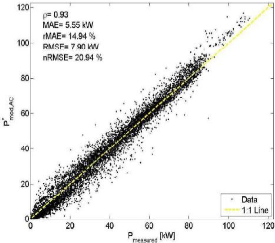
Calibrated SolarAnywhere performance, with 30-min time step, versus CSI measured output (averaged over two 15-min time steps), for 86 PV sites in 2009 in San Diego, CA
