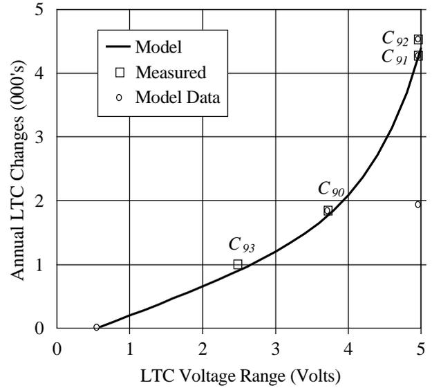
Fig. 8. Annual LTC changes versus voltage range setting.
