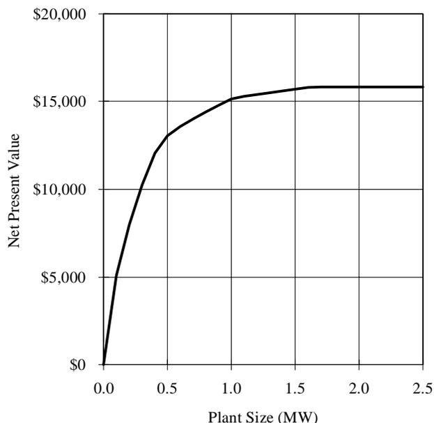
Fig. 9. LTC value versus PV plant size.
