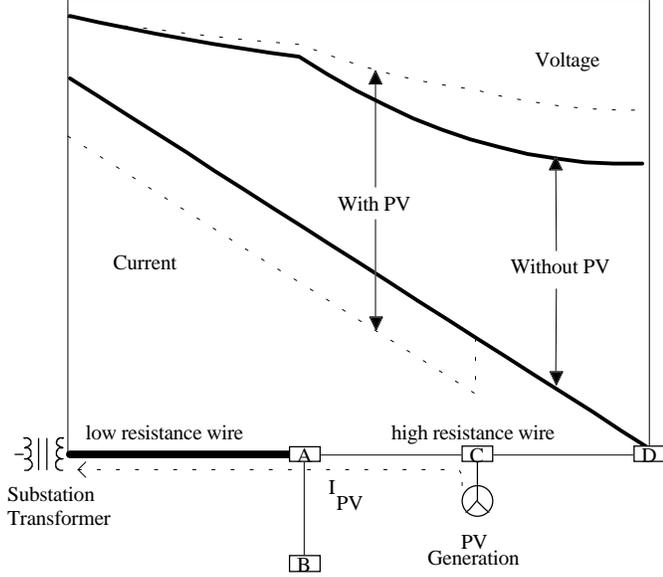
Fig. 1. Feeder voltage support provided by PV.
