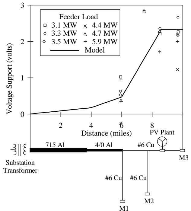
Fig. 6. Voltage support provided by PV plant at 0.40 MW output at various locations (July 6, 1993).
