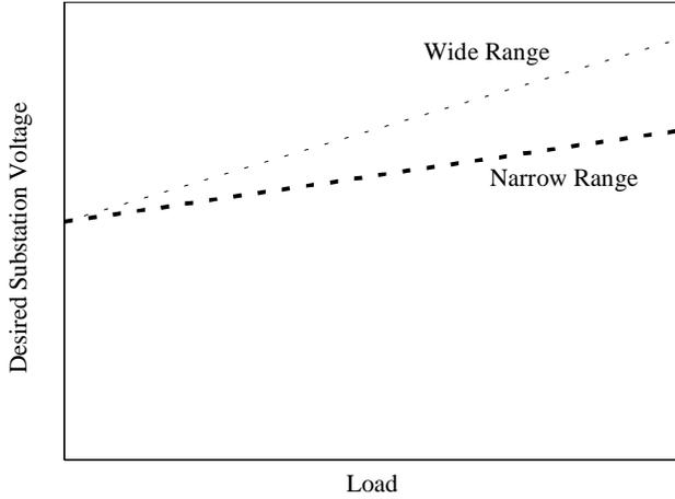
Fig. 2. Voltage versus load for two voltage range settings.
