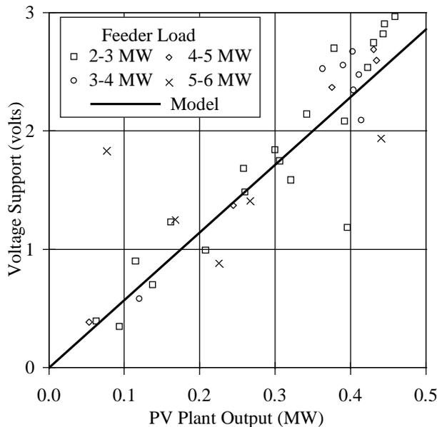
Fig. 5. Voltage support versus PV plant output at various feeder load levels (July 1, 1993 and July 6, 1993).
