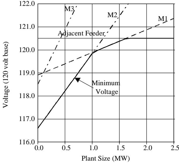
Fig. 7. Voltage support versus PV plant size.
